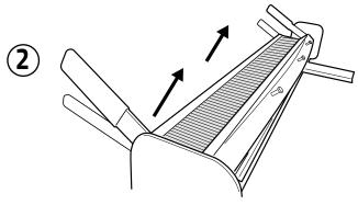
**BEND THE MESH:** Bend the mesh up or down, depending on your installation method, using a commercial or custom wooden brake.
