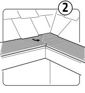
Repeat the process to install the other side of the miter, making sure the two sections meet flush at the front corner of the gutter. The mesh will overlap approximately 2 inches in the center.
