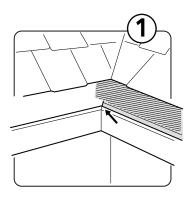
Carefully lift the front shingles and slide the back rail of the miter section underneath.
