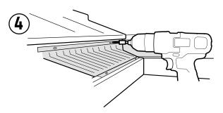
**SCREW IT DOWN:** Once both sections are in place and properly sloped, screw the front rail of each section to the front lip of the gutter, and the back rail, or mesh, to the fascia.
