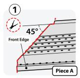
Cut the end of Piece A at 45-degrees. Next, cut a 1/2 IN.wide notch from the back wing. Then, trim off 3/4–1 IN. from the front edge in a straight line.
