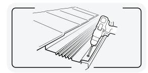
Using the provided 1/2 IN. screws, secure the front edge of the guard to the gutter at both ends using the pre-drilled screw holes (3 inches from each end). Use 2 additional screws to fasten the front edge of the guard to the gutter.
