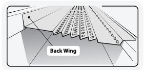
Drop the guard into the gutter with the front edge of the gutter guard resting on the front lip of the gutter. The guard is designed to rest on the gutter braces/brackets with a gradual upwards slope towards the house.
