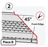
Cut the end of adjoining Piece B at 45-degrees. Repeat the 1/2 IN. wide notch cut on the back wing and the 3/4–1 IN. trim from the front edge. Pieces A & B should slightly overlap.
