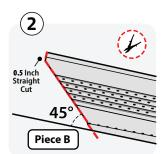
Cut the end of Piece B at 45 degrees. Next, notch the edge of the back wing in a 1/2 IN. straight line. Place Piece B atop Piece A and check that the alignment has no gapping.
