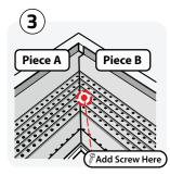
A completed inside corner should look like Image 3. Piece B should rest atop Piece A creating a seamless miter. For a tighter seal, place a screw through Piece B into Piece A to pull the pieces together.
